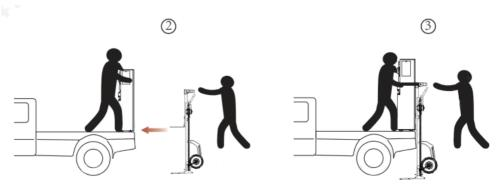
c) Use the lift to raise aPower by about 2 in. (5cm). One person pulls the dolly backward until the aPower is completely detached from the transportation; then lower the aPower to the bottom to move the aPower.
