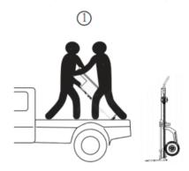
b) One person raises the platform of the dolly to the bottom position of the aPower and inserts it, and one person uses straps to tighten the aPower (if the dolly is not raised high enough, pallet can be used at the bottom of lift to pad the height).
